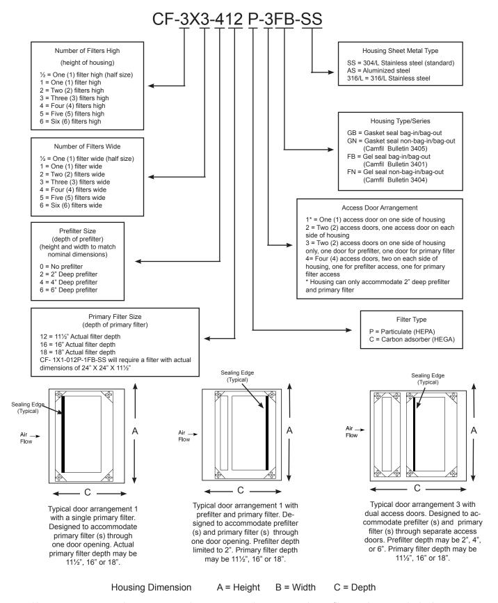
Above arrangements show upstream, downstream and upstream primary filter seals respectively. Arrangements 1 and 3 are also available with downstream primary filter seal when in-place scan testing is required.
