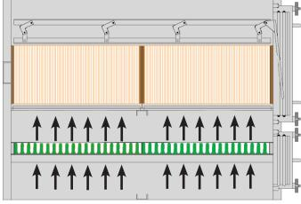
CamContain housings feature smooth surface construction. Pocket areas, that would allow contaminant build-up are minimized. All pressure retaining joints on the interior of the housing are continuously welded.
