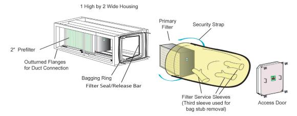
CamContain FB Housings are designed with safety in mind. Each housing is shipped with an instruction book detailing how to change the filters. The basics of filter change include installing the new filters in the change-out bag, securing the bag over the ribbed openings on the housing door opening, and performing the filter change entirely within the bag.
